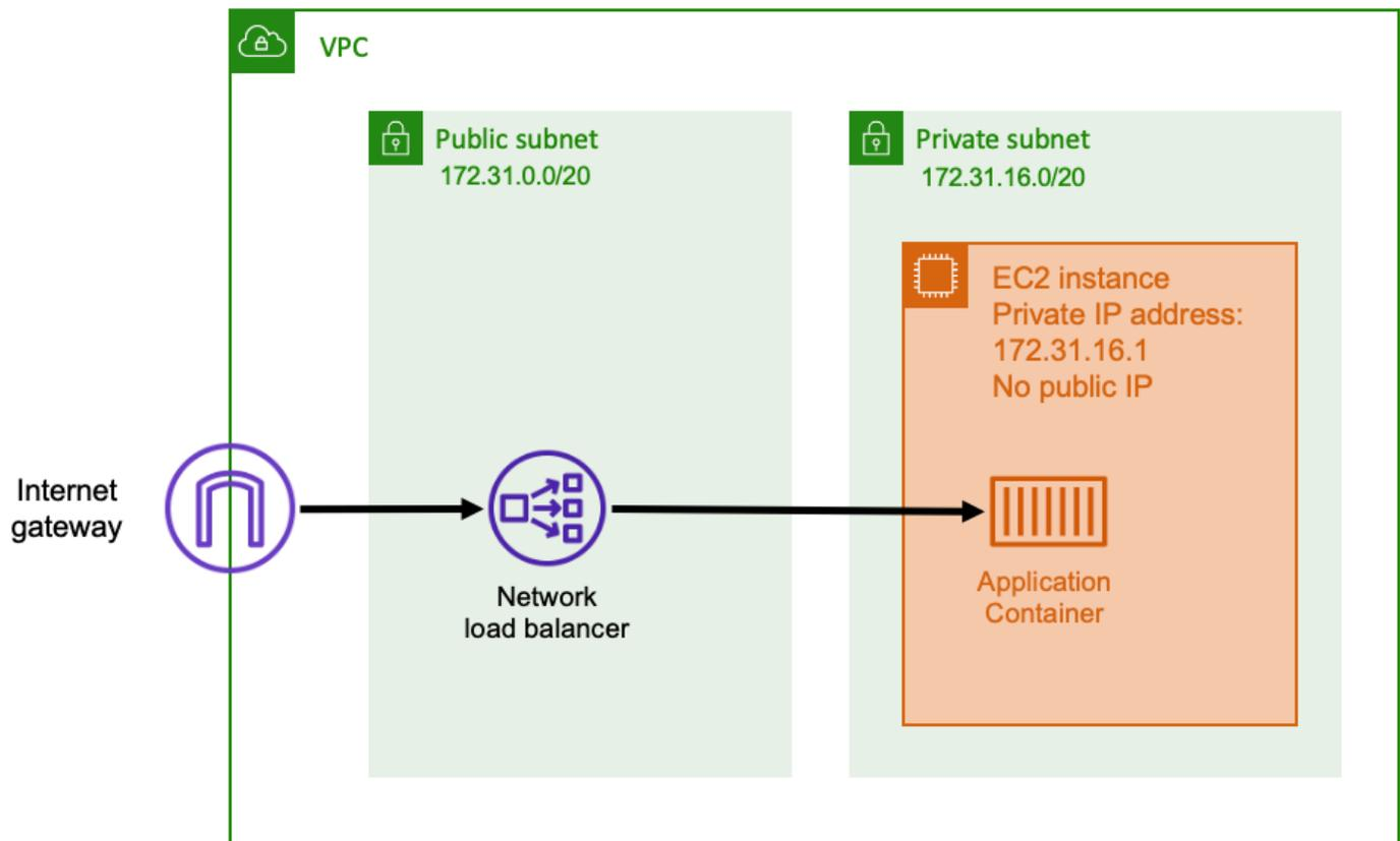
When a Network Load Balancer is used as an input, it functions similarly to an Application Load Balancer. This is because it's created in a public subnet and has a public IP address that can be accessed on the internet. The Network Load Balancer then opens a connection to the private IP address of the host running your container, and sends the packets from the public side to the private side.
