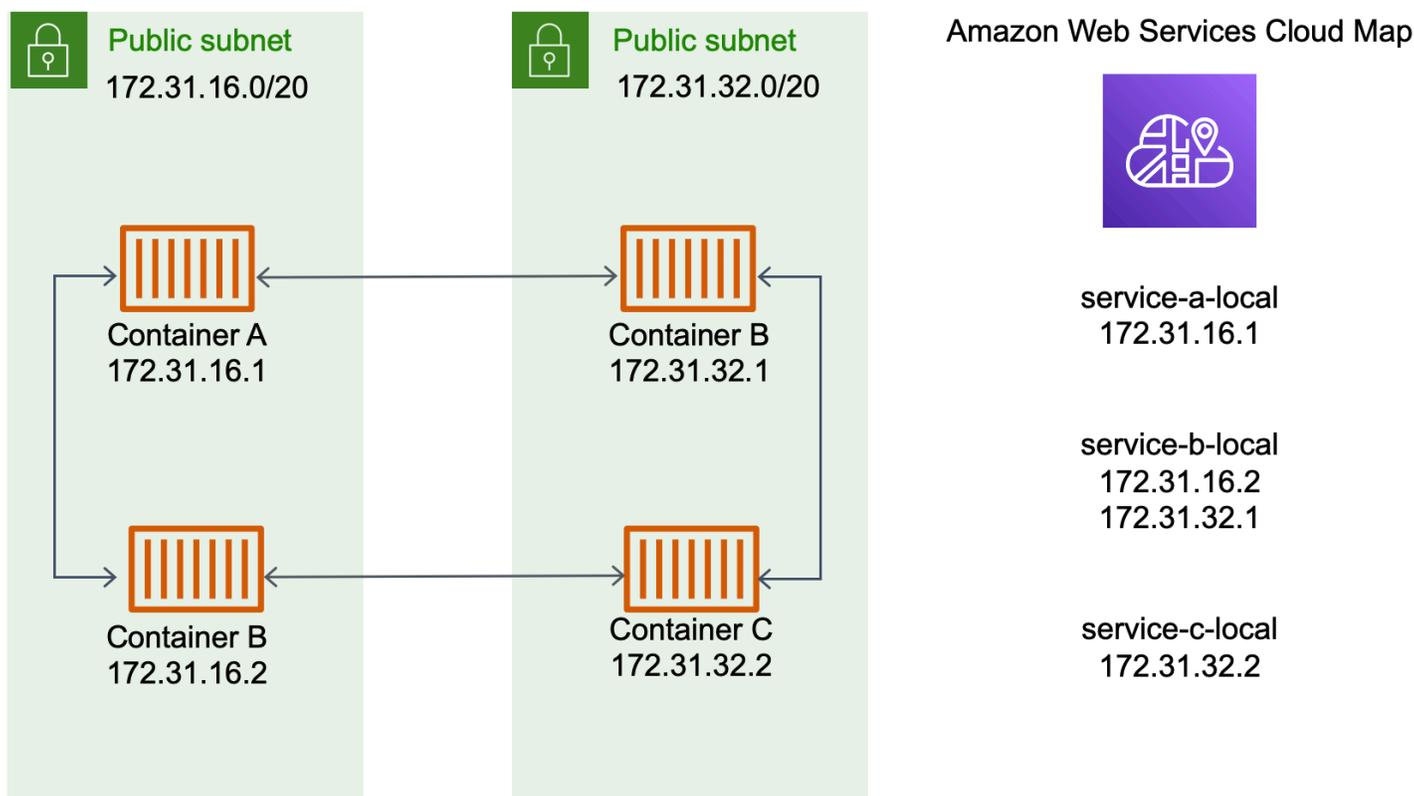
In the preceding diagram, there are three services. `service-a-local` has one container and communicates with `service-b-local`, which has two containers. `service-b-local` must also communicate with `service-c-local`, which has one container. Each container in all three of
