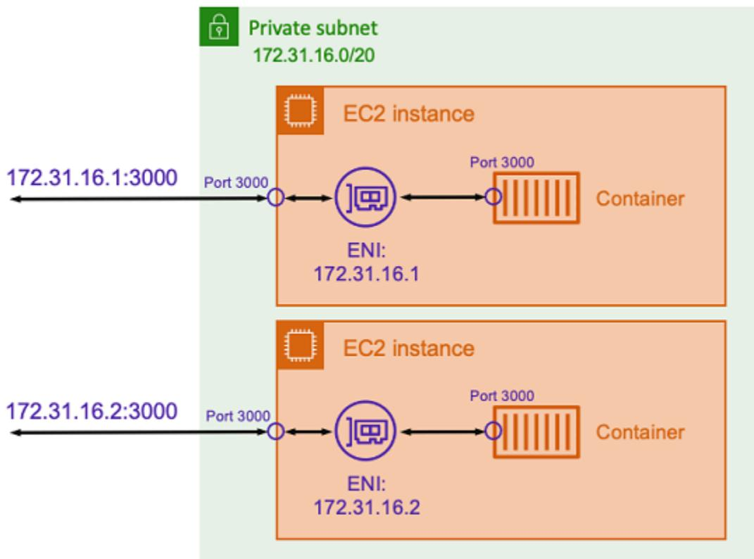
Assume that you're running a Node.js container with an Express application that listens on port 3000 similar to the one illustrated in the preceding diagram. When the host network mode is used, the container receives traffic on port 3000 using the IP address of the underlying host Amazon EC2 instance. We do not recommend using this mode.
