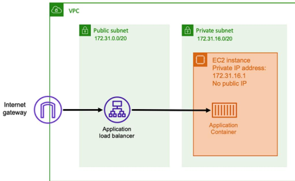
With this architecture, you create an Application Load Balancer in a public subnet so that it has a public IP address and can receive inbound connections from the internet. When the Application Load Balancer receives an inbound connection, or more specifically an HTTP request, it opens a connection to the application using its private IP address. Then, it forwards the request over the internal connection.
