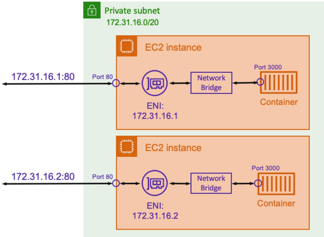
With a static port mapping, you can explicitly define which host port you want to map to a container port. Using the example above, port 80 on the host is being mapped to port 3000 on the container. To communicate to the containerized application, you send traffic to port 80 to the Amazon EC2 instance's IP address. From the containerized application's perspective it sees that inbound traffic on port 3000.
