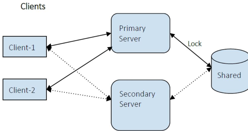
In the above diagram, a pair of messaging servers share a state by sharing file-based storage. The primary server attains the lock on the shared storage capacity, becomes active, and accepts client connections, while the secondary server remains in passive mode. Meanwhile, the primary and secondary servers will be made aware of one another's status via periodic, heartbeat pings.
