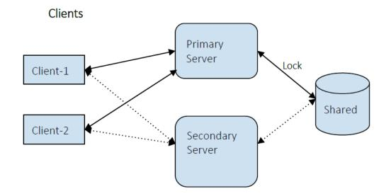
In the above diagram, a pair of messaging servers share a state by sharing file-based storage. The primary server attains the lock on the shared storage capacity, becomes active, and accepts client connections, while the secondary server remains in passive mode. Meanwhile, the primary and secondary servers will be made aware of one another's status via periodic, heartbeat pings.
