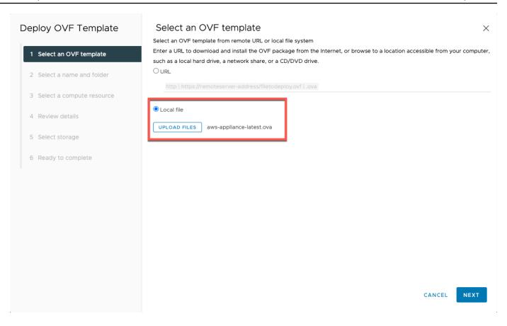
Follow the deployment wizard steps to deploy it. On the Select storage page, select virtual disk format Thick Provision Lazy Zeroed.
