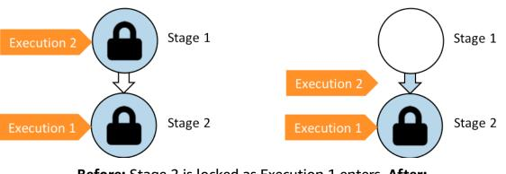
**Before:** Stage 2 is locked as Execution 1 enters. **After:** Execution 2 exits Stage 1 and waits between stages.
