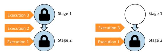
**Before:** execution 2 waits between stages while execution 3 enters stage 1. **after:** execution 3 exits stage 1. execution 2 is superseded by execution 3.
