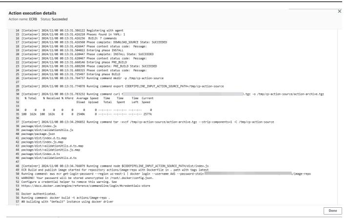
16. Troubleshoot any failed actions. For example, the ECS deploy action can fail if the imagedefinitions.json file is not in the source repository. The following is an example of the error message that displays when the imagedefinitions.json file is missing.
