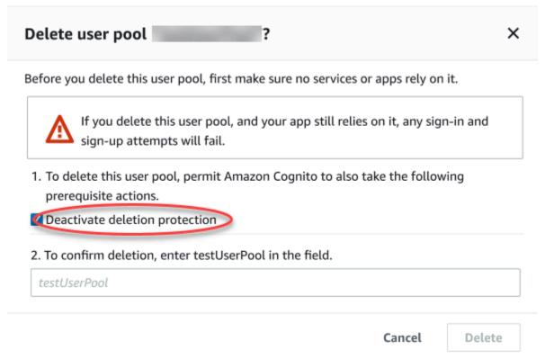
When you want to delete a user pool with an Amazon Cognito API request, you must first change DeletionProtection to Inactive in an <u>UpdateUserPool</u> request. If you don't deactivate deletion protection, Amazon Cognito returns an InvalidParameterException error. After you deactivate deletion protection, you can delete the user pool in a <u>DeleteUserPool</u> request.
