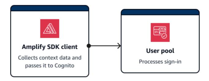
Amplify SDKs support mobile clients that authenticate with Amazon Cognito directly. Clients of this kind make direct API requests to Amazon Cognito public API operations. Amplify clients automatically collect context data for threat protection by default.
