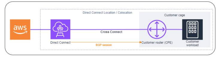
Extend the Direct Connect connection at Layer 2 (data link layer) via a "circuit" from the Direct Connect location to the customer location by working with Direct Connect Partners. The router installed at the customer location will directly form a BGP session with the Amazon equipment. For example, technologies that can be used are Metro Ethernet, Dark Fibre, or Wavelength. The following shows an example of this Direct Connect connectivity option.
