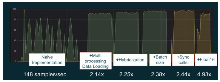
Example GPU performance optimizations. Chart source: Performance Tricks with MXNet Gluon
