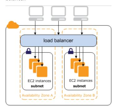
The DNS name of an internal load balancer is publicly resolvable to the private IP addresses of the nodes. Therefore, internal load balancers can only route requests from clients with access to the VPC for the load balancer. For more information, see *Internal load balancers*.
