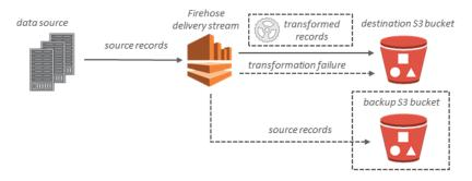
For Amazon Redshift destinations, streaming data is delivered to your S3 bucket first. Amazon Data Firehose then issues an Amazon Redshift **COPY** command to load data from your S3 bucket to your Amazon Redshift cluster. If data transformation is enabled, you can optionally back up source data to another Amazon S3 bucket.
