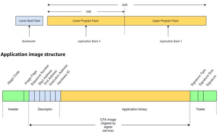
The diagram shows the primary components of the application image stored on each bank of the device.
