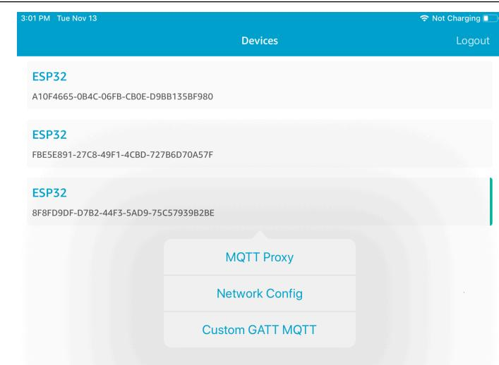
4. After you choose **Network Config** for your board, the microcontroller sends a list of the networks in the vicinity to the mobile device. Available Wi-Fi networks appear in a list under **Scanned Networks**.
