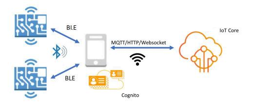
Using the Mobile SDKs for FreeRTOS Bluetooth Devices, you can write native mobile applications that communicate with the embedded applications on your microcontroller over BLE. For more information about the mobile SDKs, see <u>Mobile SDKs for FreeRTOS Bluetooth devices</u>.
