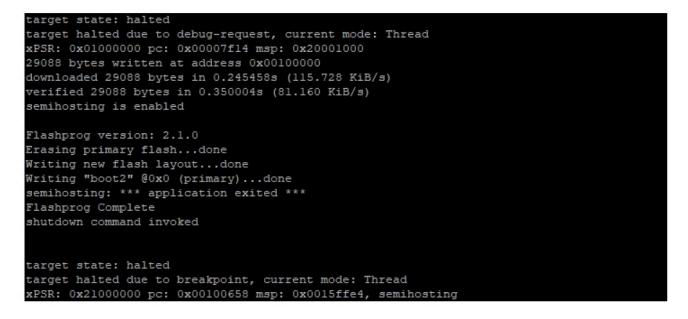
b. The firmware uses the Wi-Fi chipset for its functionality, and the Wi-Fi chipset has its own firmware that must also be present in the flash. You use the flashprog.py utility to flash the Wi-Fi firmware in the same way that you did to flash the Boot2 boot-loader and the MCU firmware. Use the following commands to flash the Wi-Fi firmware.
