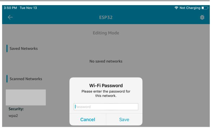
The microcontroller connects to and saves the network. The network appears under **Saved Networks**.
