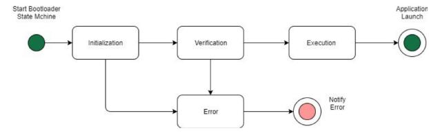
The bootloader process is shown in the following state machine.
