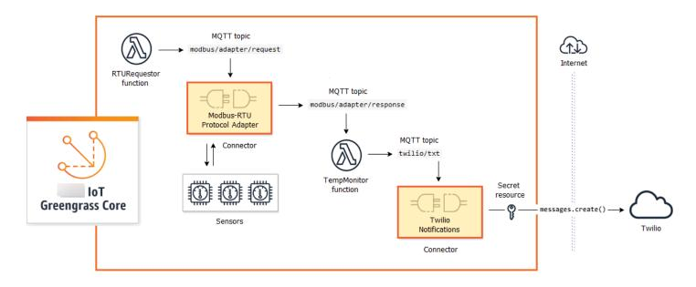
Solutions often include user-defined Lambda functions that sit next to connectors and process the data that the connector sends or receives. In this example, the TempMonitor function receives data from Modbus-RTU Protocol Adapter, runs some business logic, and then sends data to Twilio Notifications.
