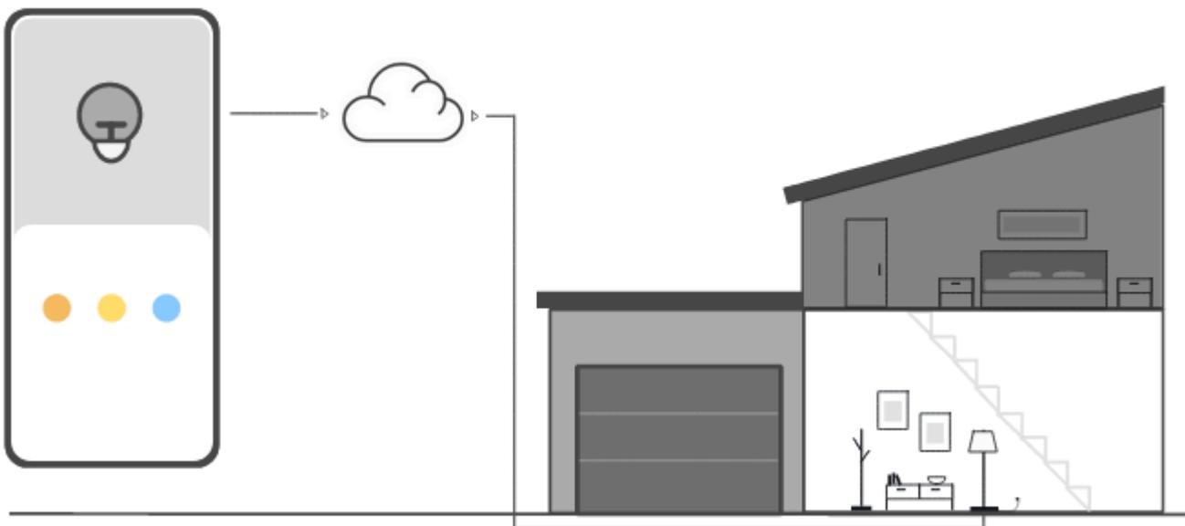
The animation in this step shows how two devices, the control device on the left and a smart lamp in the house on the right, connect and communicate with Amazon IoT Core in the cloud. The animation shows the devices communicating with Amazon IoT Core and reacting to the messages they receive.
