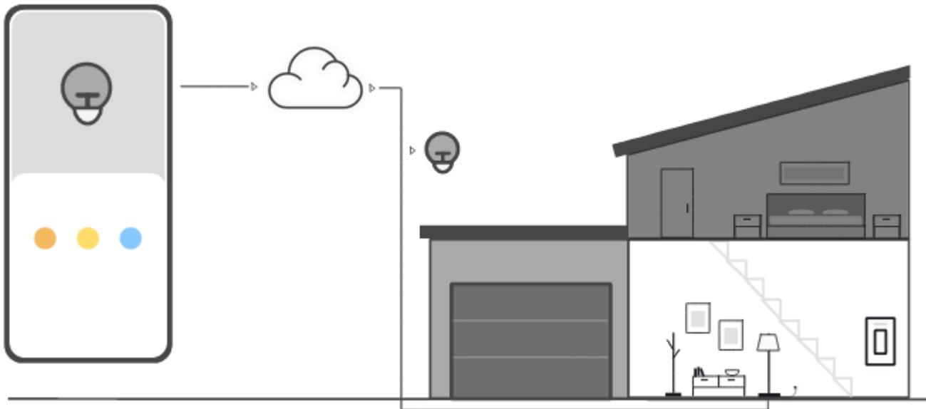
The animation in this step shows how the Device Shadow service in Amazon IoT Core saves device state information for the control device and the smart lamp. While the smart lamp is offline, the Device Shadow saves commands from the control device.
