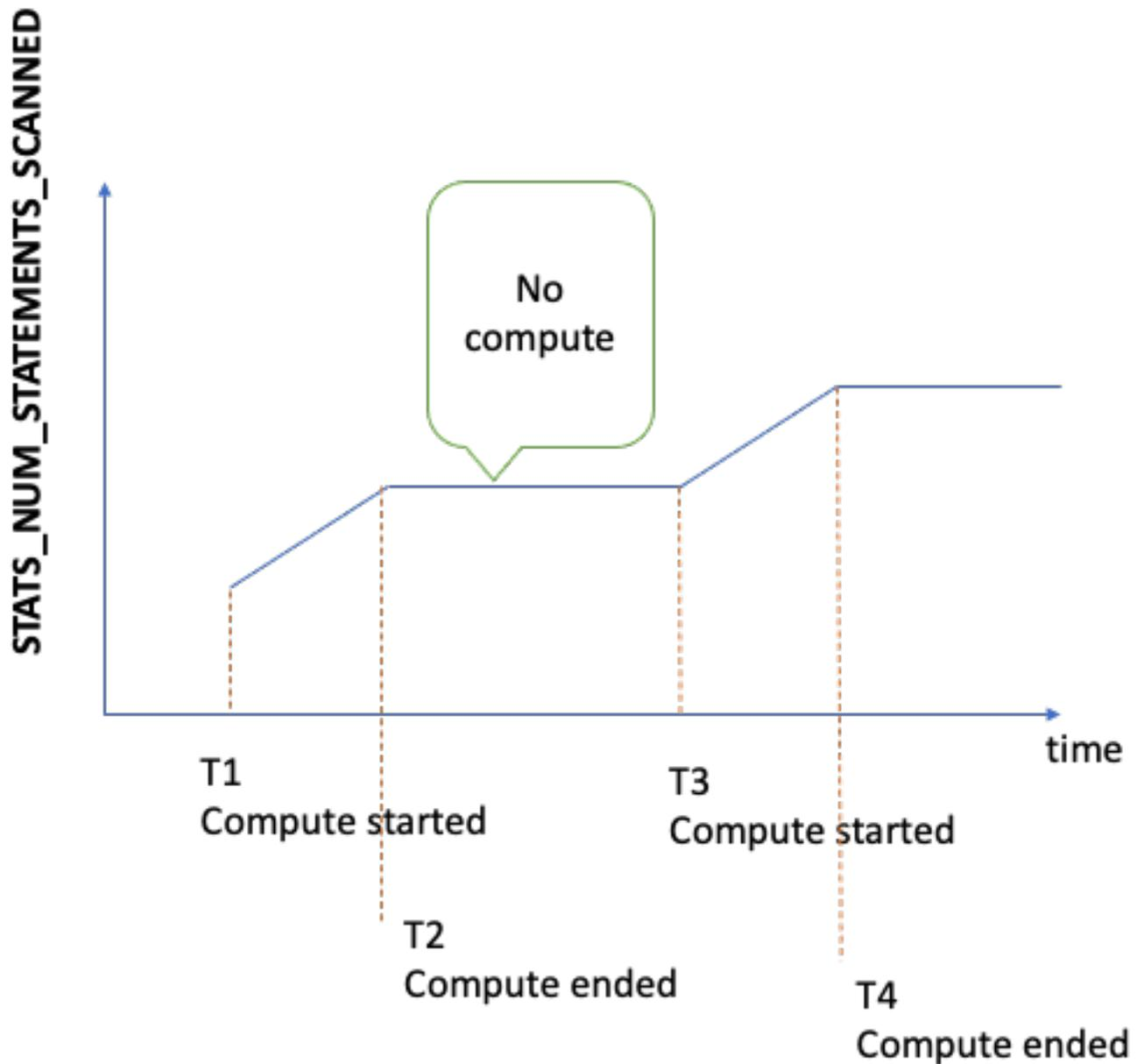
When computation is happening, the slope of the graph shows you how fast (the steeper the slope, the faster statistics are being computed).
