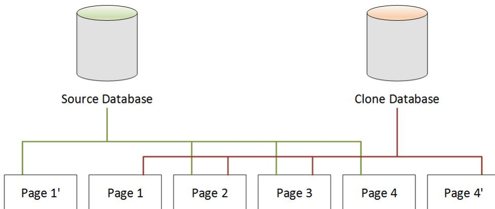
As shown in the second scenario, after DB cloning, there is no additional storage required at the point of clone creation. However, as changes occur in the source database and clone database, only the changed pages are created, as shown in the third and fourth scenarios. As more changes occur over time in both the source database and clone database, you need incrementally more storage to capture and store the changes.
