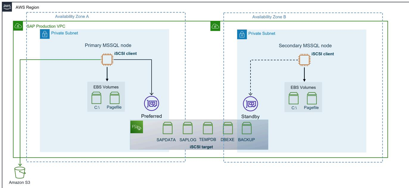
FSx for ONTAP supports both, iSCSI and SMB protocol to be used for SQL server deployments on Amazon. The iSCSI protocol works at the block level, and is expected to drive higher performance for SQL server with OLTP-type workloads than the same system configured with SMB. We recommend configuring your MSSQL on FSx for ONTAP using the iSCSI protocol.
