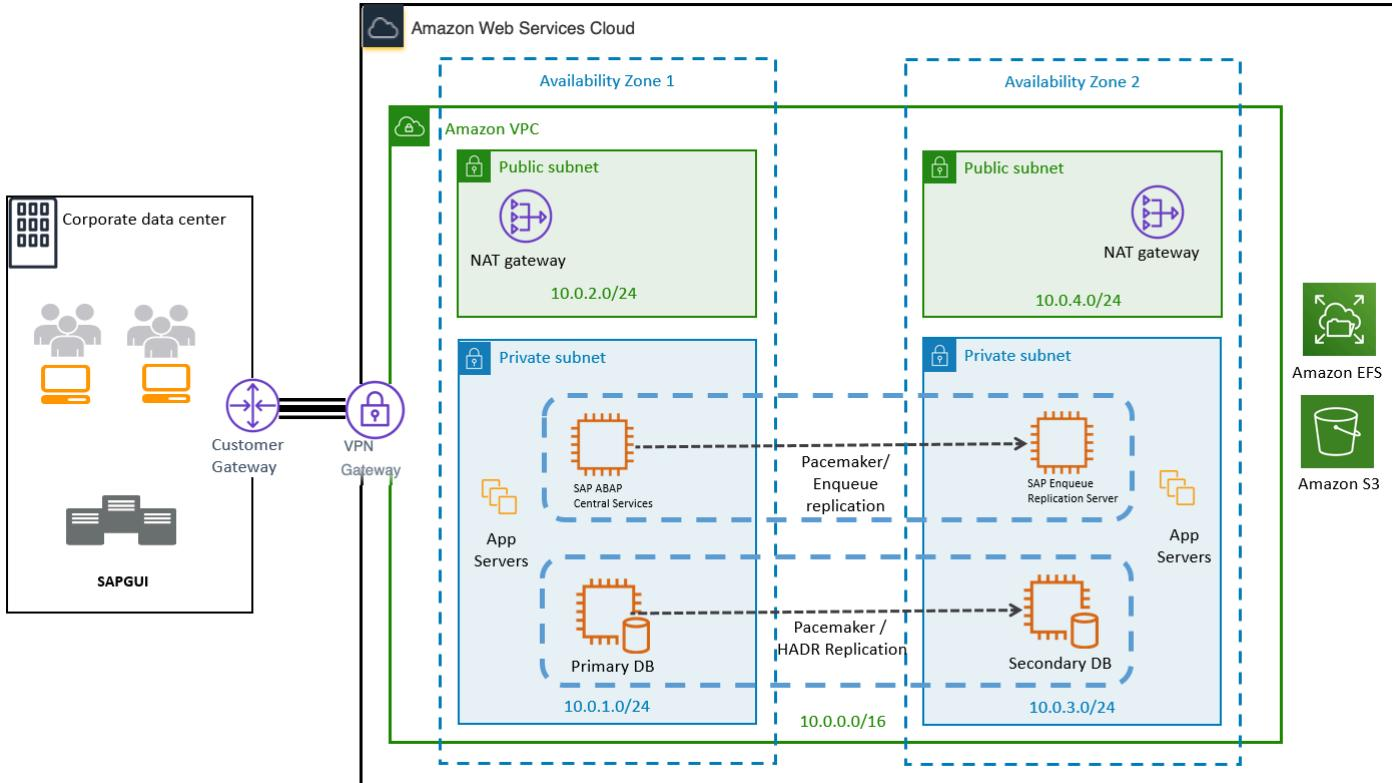
Figure 1 – High-level HA architecture for SAP with IBM Db2 on Amazon
