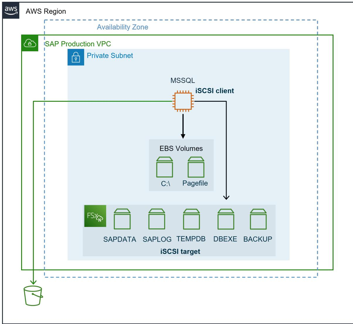
The following diagram presents a high availability setup for MSSQL database with FSx for ONTAP.
