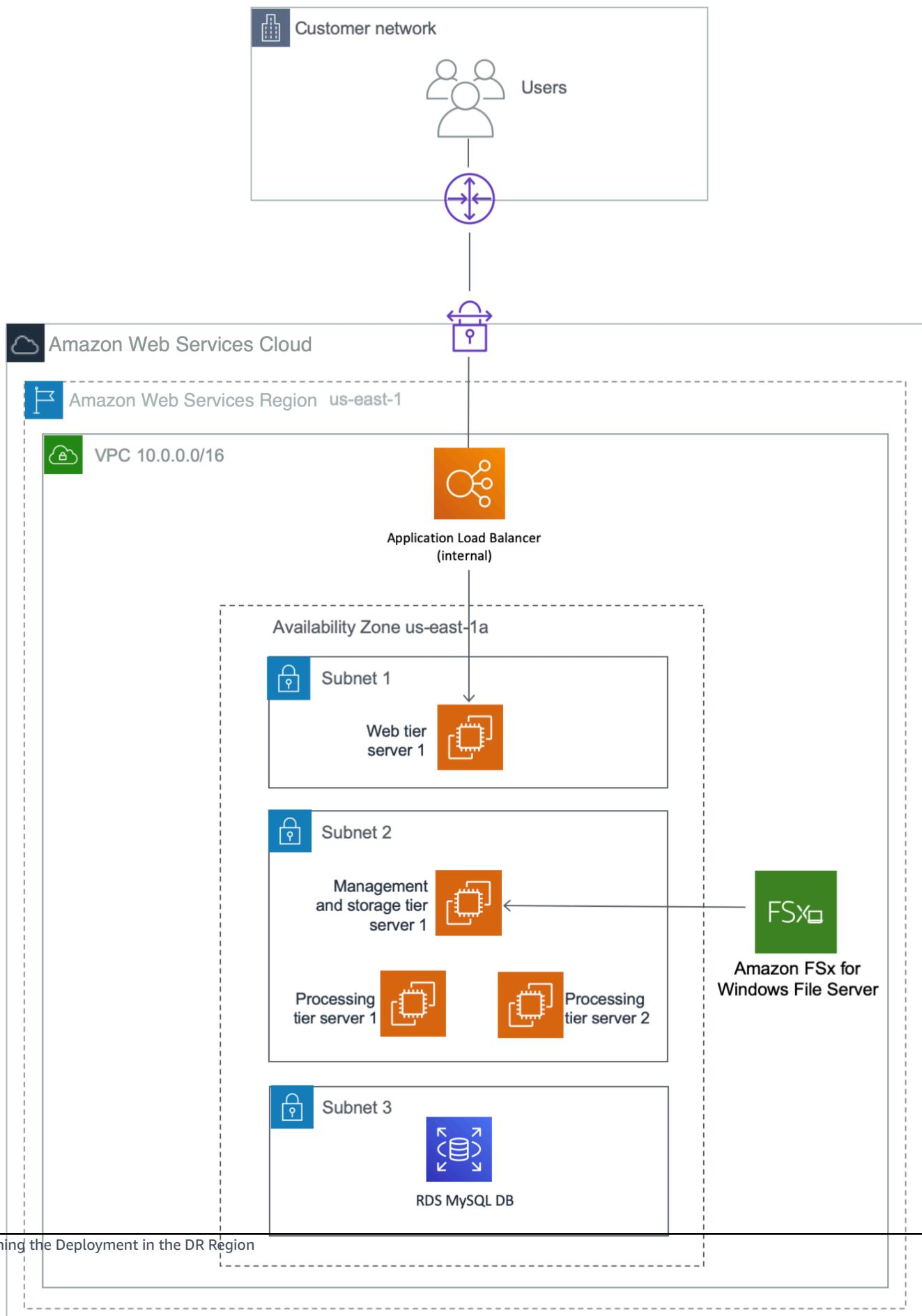
Figure 4 shows the user connectivity using Route 53 as an example. You can also use your own DNS. During normal operations, the value of the CNAME record for SAP BusinessObjects BI Platform points to the Application Load Balancer of the primary region. The load balancer distributes the load between the available web servers that deploy the SAP BusinessObjects BI Platform web applications.
