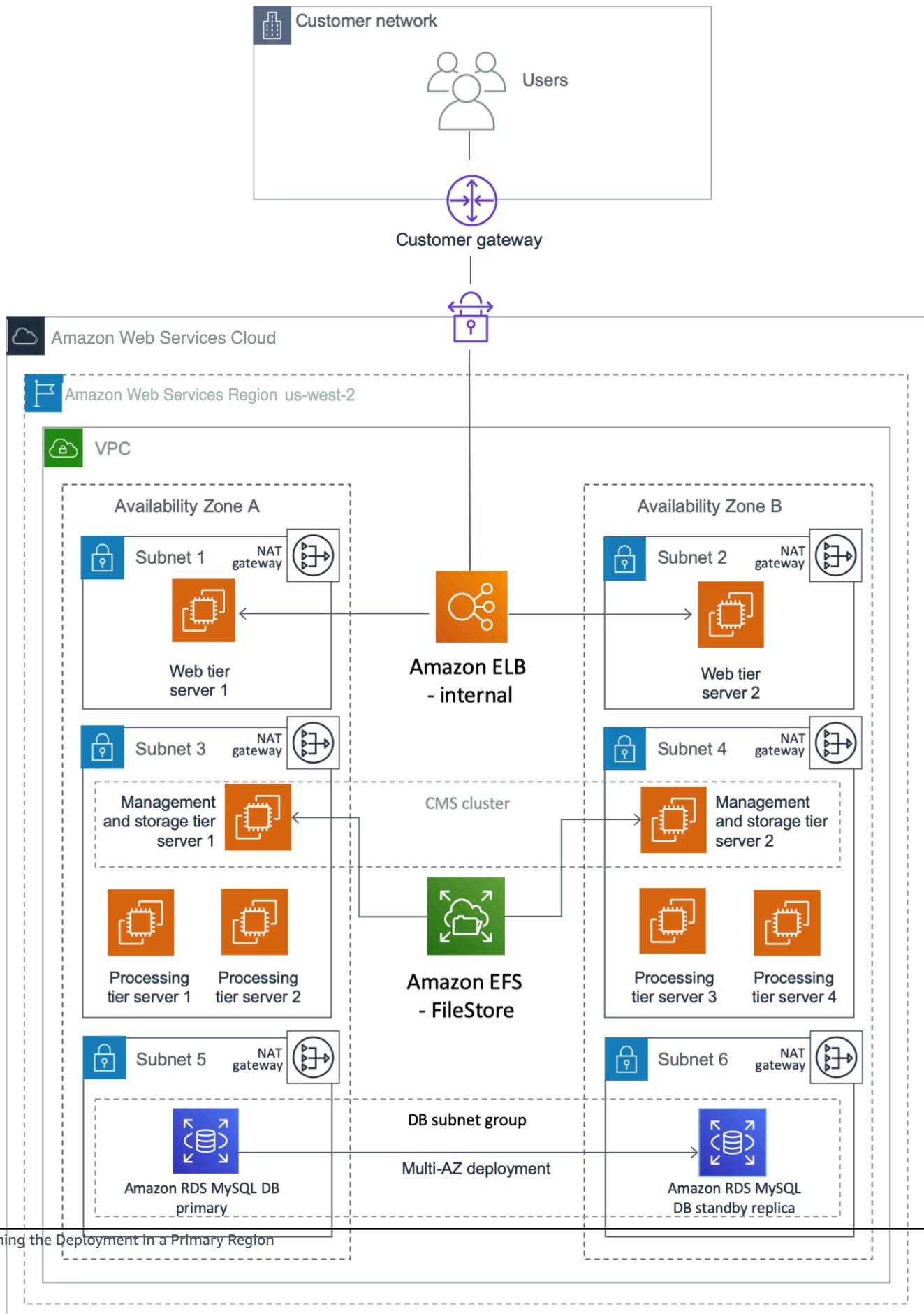
This example puts the web tier in a dedicated subnet. End users will access the web tier servers where the web applications are deployed. You can use security groups to restrict connectivity between the subnets only to the required ports. For example, you can restrict connectivity from the application subnet to the database subnet to allow access only to the database listener port. The Multi-AZ architecture provides both load balancing and HA.
