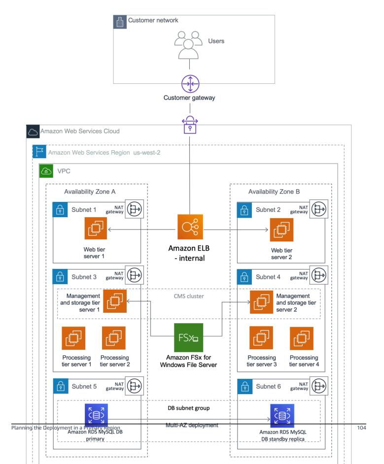
This example puts the web tier in a dedicated subnet. End users will access the web tier servers where the web applications are deployed. You can use security groups to restrict connectivity between the subnets only to the required ports. For example, you can restrict connectivity from the application subnet to the database subnet to allow access only to the database listener port. The Multi-AZ architecture provides both load balancing and HA.
