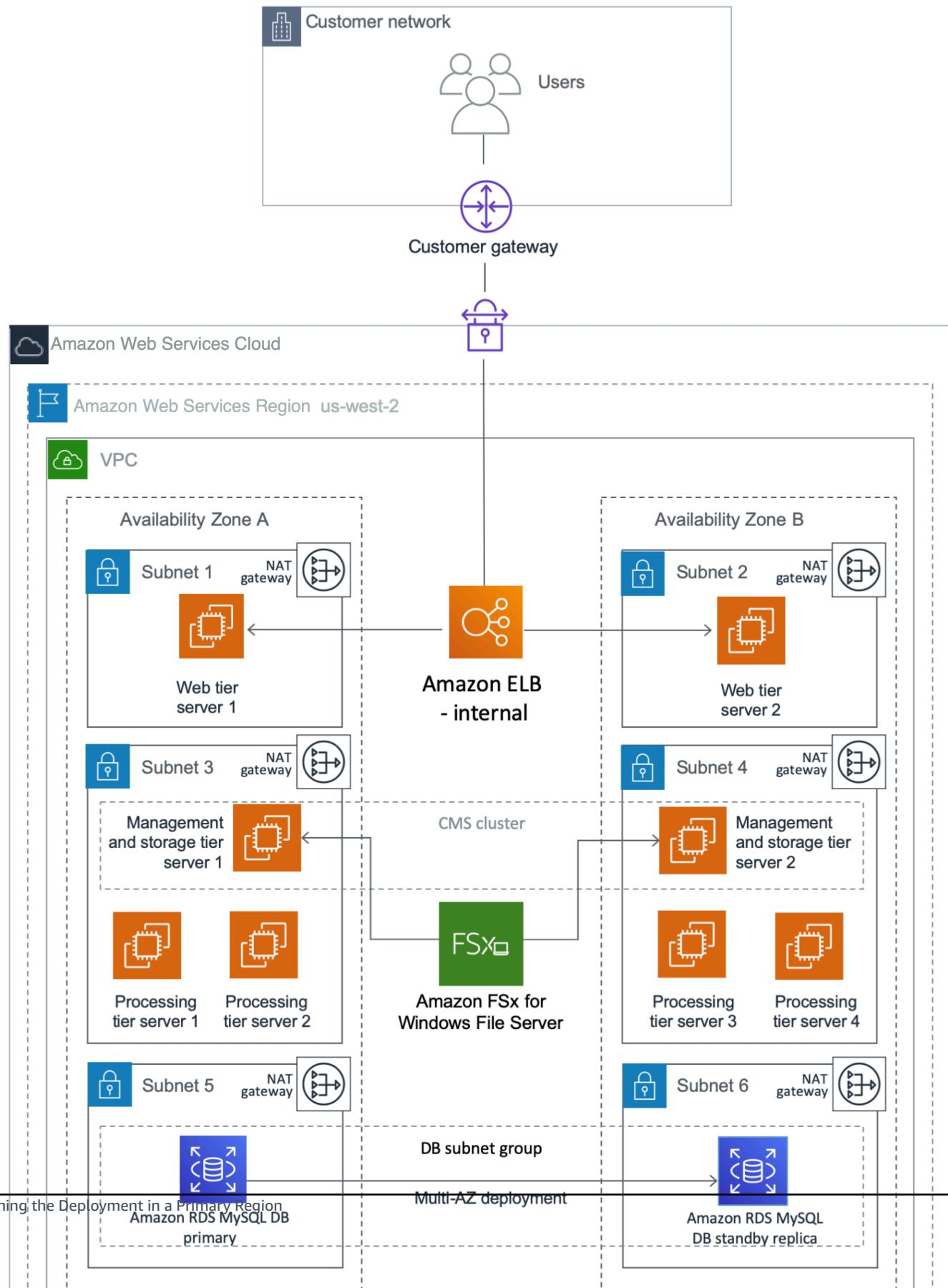
This example puts the web tier in a dedicated subnet. End users will access the web tier servers where the web applications are deployed. You can use security groups to restrict connectivity between the subnets only to the required ports. For example, you can restrict connectivity from the application subnet to the database subnet to allow access only to the database listener port. The Multi-AZ architecture provides both load balancing and HA.
