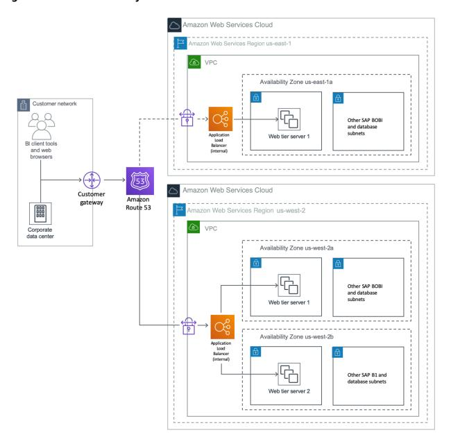
In the event of DR or when performing a DR drill, you can either manually switch the DNS to point to the DR region or you can use automatic failover by using Route 53 health checks. For details, see <a href="Configuring DNS Failover">Configuring DNS Failover</a> in the Route 53 documentation. Redirect all the users to the DR region as shown in Figure 5.
