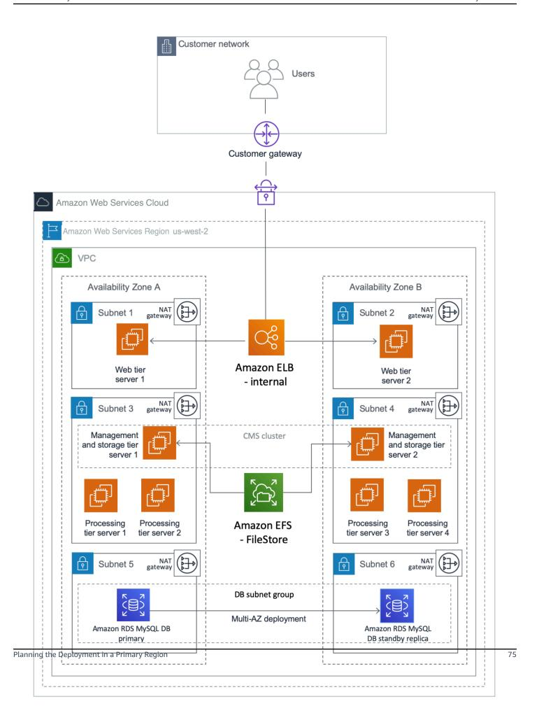
This example puts the web tier in a dedicated subnet. End users will access the web tier servers where the web applications are deployed. You can use security groups to restrict connectivity between the subnets only to the required ports. For example, you can restrict connectivity from the application subnet to the database subnet to allow access only to the database listener port. The Multi-AZ architecture provides both load balancing and HA.
