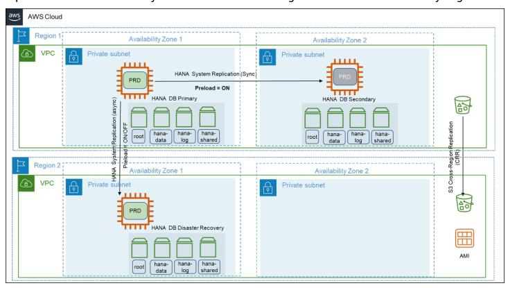
The following diagram shows a multi-tier replication where the replication is configured in a chained fashion.
