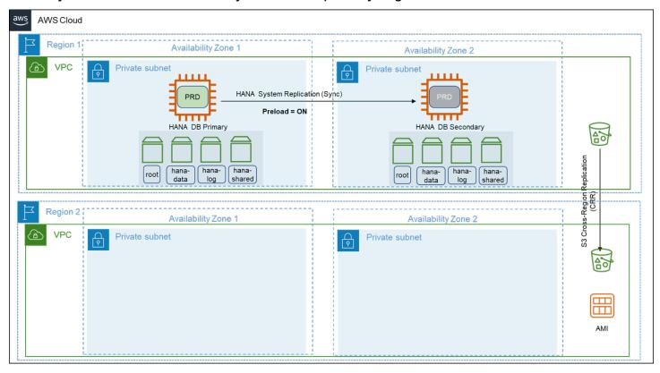
Pattern 6: Primary Region with two Availability Zones for production and secondary Region with compute and storage capacity deployed in a single Availability Zone
