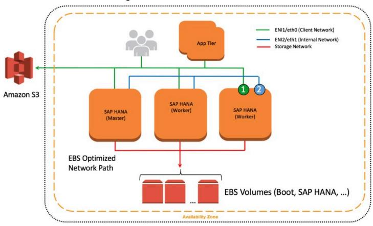
Figure 10: Network interfaces attached to SAP HANA nodes
