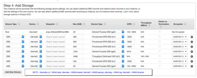
Figure 3: SAP HANA Storage Configuration with the console
