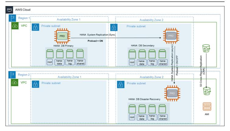
Pattern 7: Primary Region with two Availability Zones for production and a secondary Region with compute and storage capacity deployed, and data replication across two Availability Zones
