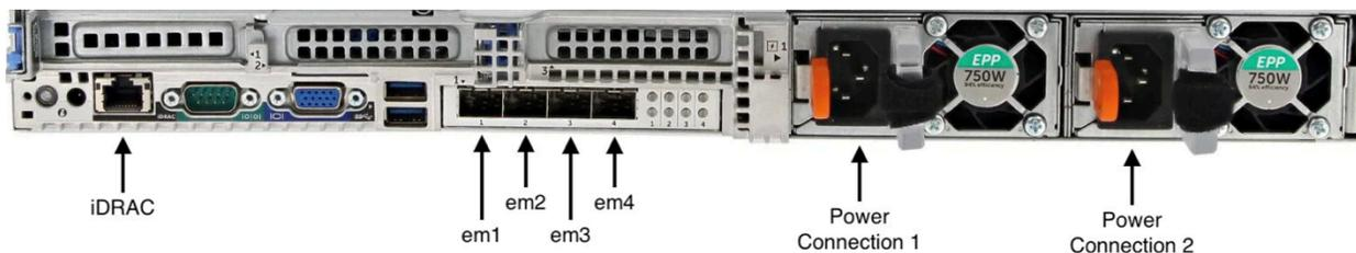
hardware appliance one rear with network and power connector labels.
