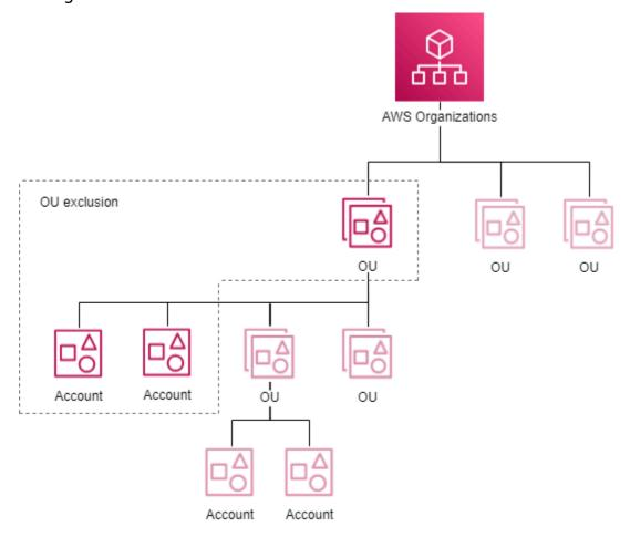
The second diagram shows the impact of adding an organization unit (OU) exclusion on a parent OU and all child OUs. As a result, IPAM will not manage the IP addresses in accounts in the parent OU or in accounts in any child OUs. IPAM will manage the IP addresses in accounts in the OUs outside of the exclusion.
