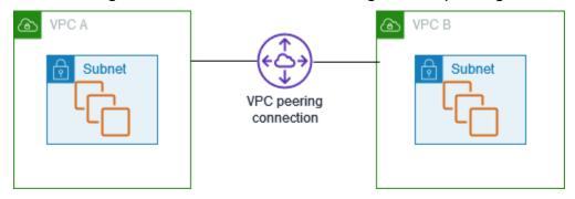
Amazon uses the existing infrastructure of a VPC to create a VPC peering connection; it is neither a gateway nor a VPN connection, and does not rely on a separate piece of physical hardware. There is no single point of failure for communication or a bandwidth bottleneck.
