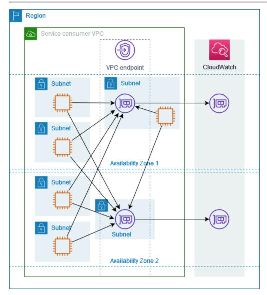
If it's better for your use case, you can send traffic from your resources to the Amazon Web Services service by using the endpoint network interface in the same Availability Zone. To do so, use the private zonal endpoint or IP address of the endpoint network interface.
