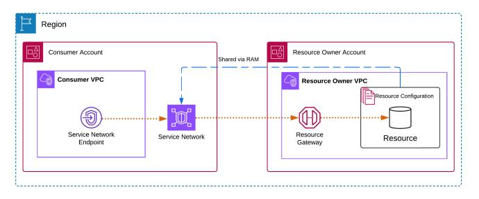
Network connections can only be initiated from the VPC that has the service-network endpoint to the resources and services in the service network. The VPC with the resources and services can't initiate network connections into the endpoint VPC.
